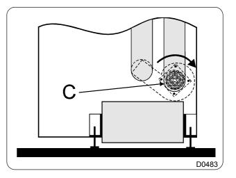
If it is rotating in the wrong direction, invert two of the three phases on the power supply isolating switch to reverse the direction of rotation of the fan.
