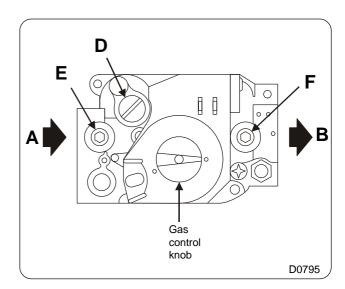
1/ Close the gas inlet and remove the binding screw from the pressure tapping (F) and connect the manometer tube.
