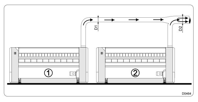
The indicated evacuation diameter is the dryer outlet diameter.
