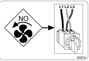
Check again the direction of rotation of the fan then replace the hose and its collar.
