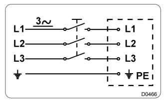
Pass the machine power supply cable through the orifice (see sketch).
