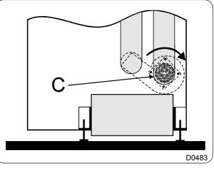
If it is rotating in the wrong direction, invert two of the three phases on the power supply isolating switch to reverse the direction of rotation of the fan.
